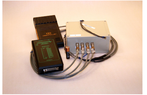
FIG. 6. (color online) Portable, low-power prototype, scale shown with AA batteries. The computer is in the black and yellow box, while the AD converter is in the black and green box. The interconnection between the AD converter and filter/amplifier box still needs to be adjusted.
