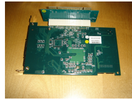
(c) Reiser module and A/D-board combined
