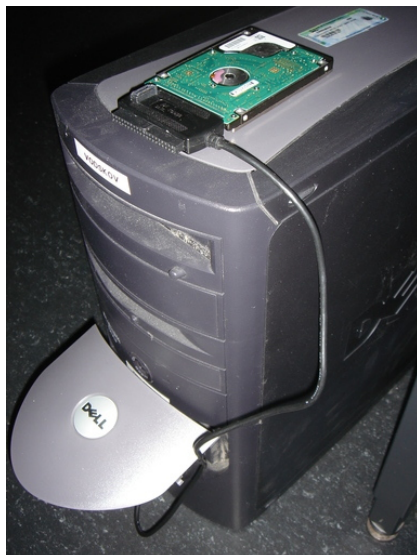
Figure 9.1: Picture of 2.5” IDE hard disk connected through USB
